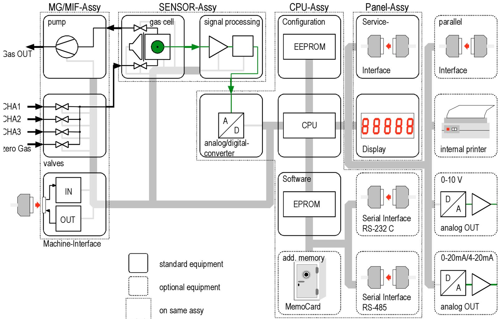
Fig. 5 Equipment Components Diagram
