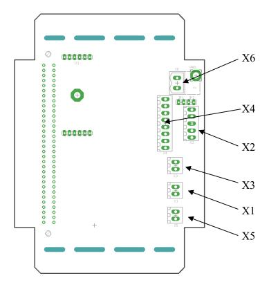
Fig. 12 Electrical connectors / Rear view
