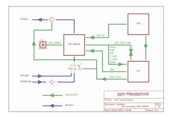
Fig. 5 PLC or plant connection
